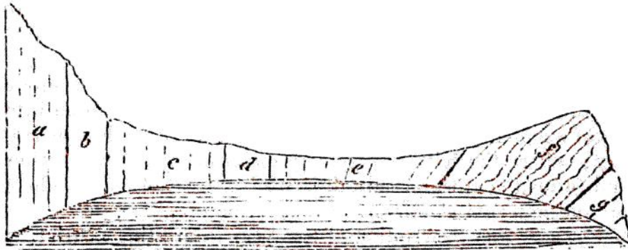
a. Chalk. b. Chalk marle. c. Green sand. d. Blue marle. e. Iron sand. f. Purbeck beds. g. Portland beds.
