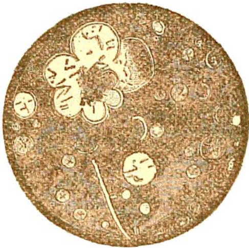
Fig. 21.—Clastic Structure, of Inorganic origin—Section of a Piece of Greywacke. (10 Diameters. See p. 232.)
