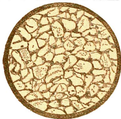
Fig. 38.—Microscopic Structure of Quartzite. (Magnified 20 diameters.)
