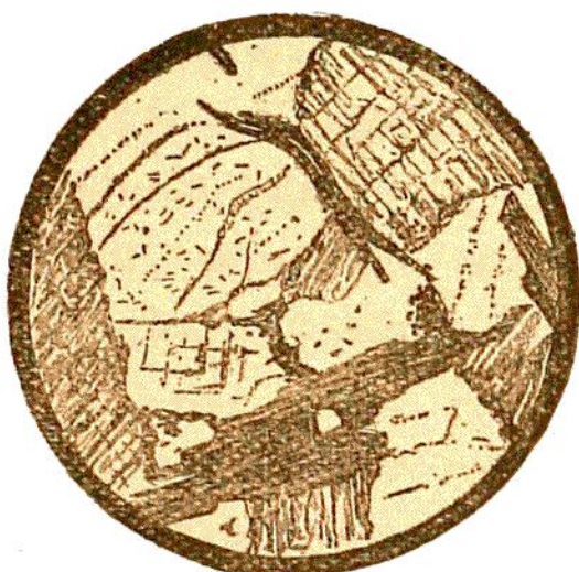
Fig. 15.—Holocrystalline Structure. Granite (20 Diameters). The white portions are Quartz, the striped parts Feldspar, the long, dark, finely striated stripes are Mica. (See p. 273.)
