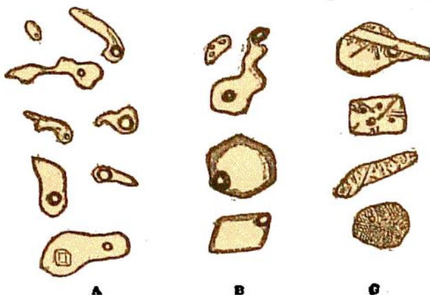
Fig. 11.—Cavities in Crystals, highly magnified; A, Liquid Inclusions; B, Glass Inclusions; C, Cavities showing the devitrification of the original glass by the appearance of crystals, etc., until in the lowest figure a stony or lithoid product is formed.
