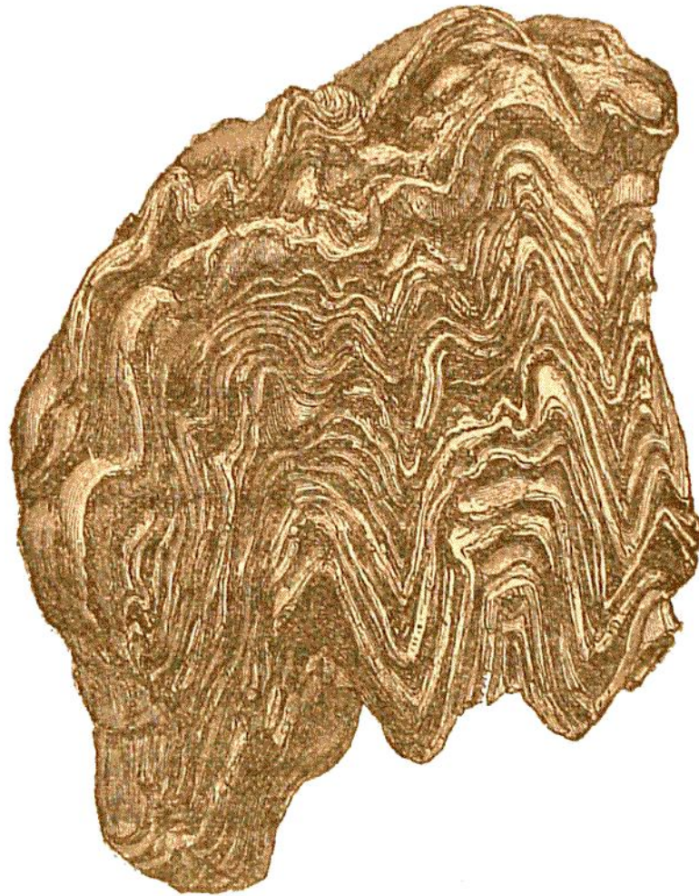
Fig. 36.—View of a hand-specimen of contorted mica-schist, two-thirds natural size. (B. N. Peach.)
