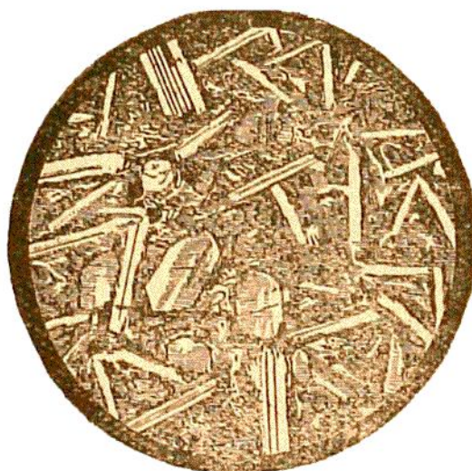
Fig. 16.—Hemi-crystalline Structure. Dolerite, consisting of a triclinal Feldspar, Augite, and Magnetite in a devitrified Ground-mass (20 Diameters). The numerous narrow prisms are triclinal Feldspar; the broader monoclinic forms, slightly shaded in the drawing, are Augite; the black specks are Magnetite; the needle-shaped forms are Apatite. (See p. 294.)
