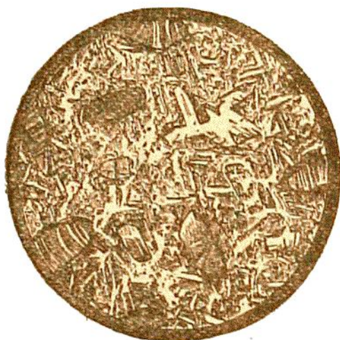
Fig. 32.—Microscopic Structure of Basalt (magnified). The large shaded crystals are Olivine considerably serpentinized; the numerous small white prisms are Plagioclase. A few Augite prisms occur which, to the right of the centre of the drawing, are aggregated into a large compound crystal. The black specks are Magnetite.
