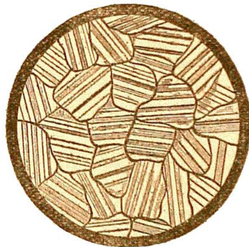
Fig. 28.—Microscopic Structure of white Statuary Marble. (Magnified 50 Diameters.)
