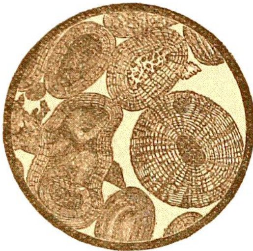
Fig. 27.—Microscopic Structure of Oolitic Limestone, after Sorby. (Magnified 30 Diameters.)
